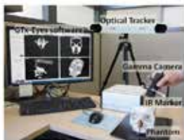
Figure 1: The FreeSPECT prototype system integrates compact gamma camera, optical tracker, and in-house GTxEyes software platform.
