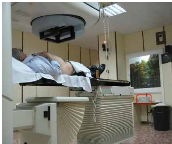
Figure 1. Experimental setup for patient organ neutron dose estimation in the treatment room. Detector location is marked in red.
