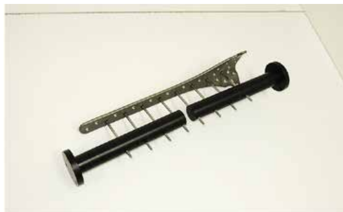
Fig. 1. Model of a novel plate external fixation with simulated tibia fragments apart.
