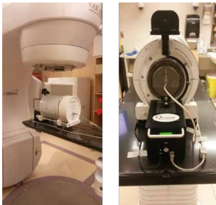
Figure 1. The QUASAR™ Cylindrical Motion Insert (with A1SL chamber) for the ArcCHECK™ phantom.
