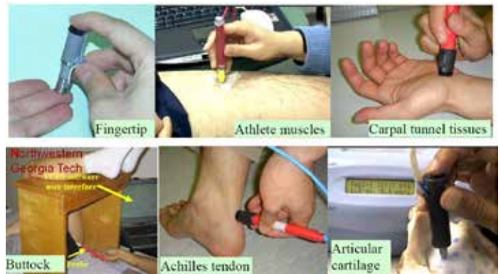
Figure 1. Assessment of musculoskeletal tissue biomechanical properties using tissue ultrasound palpation sensor (TUPS).
