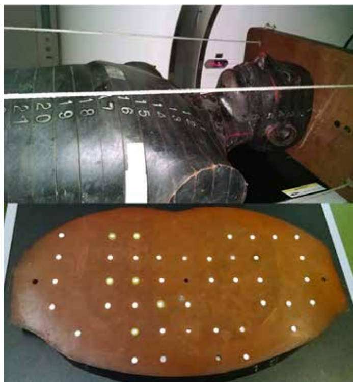
Figure 1– Adult anthropomorphic phantom positioned inside the gantry (above); positions of the dosimeter-holders (in green) inside slice 15 (below).
