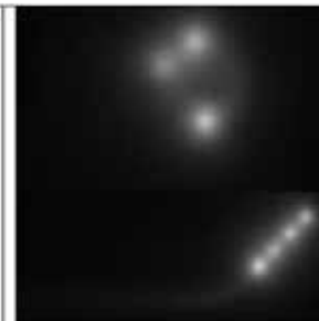
Figure 1c: Illustration of dwell positions used for analysis, produced by irradiation of Ir-192 HDR source.
