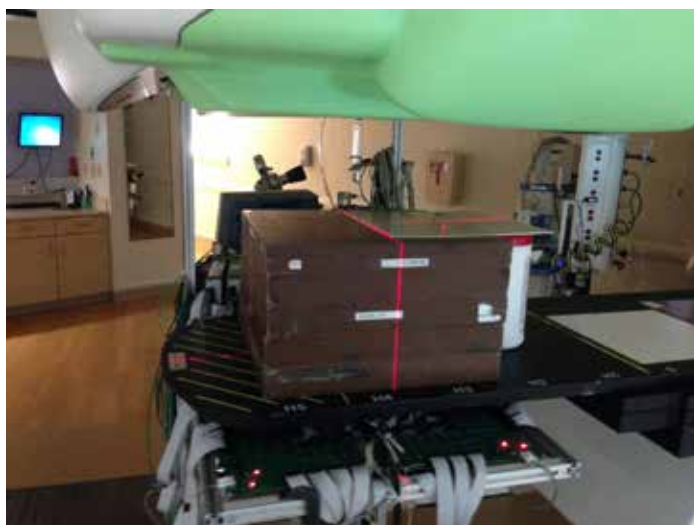
Figure 2: A radiography experiment in which the edge of a 1 mm piece of solid water on top of a 24 cm stack is imaged.
