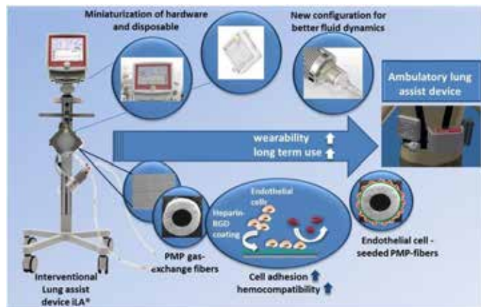
Fig1: transformation of the iLA ® to a longterm ambulatory lung assist device.
