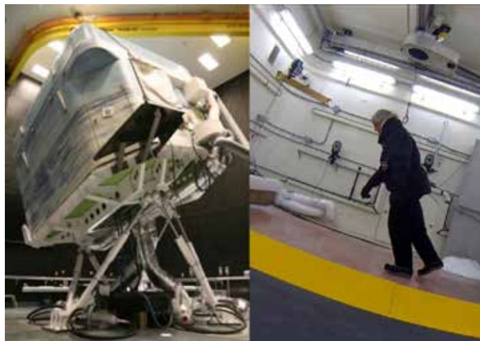
Figure 1. WinterLab being used to test footwear slip resistance on ice.
