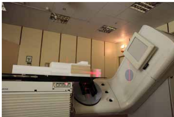
Figure 2. Anthropomorphic phantom used to generate the equivalent neutron and photon dose estimation models.
