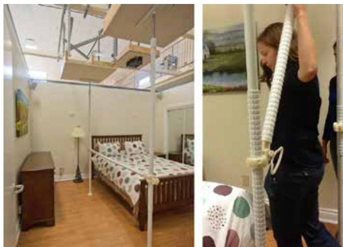
Figure 2. HomeLab being used to test the MoveEasy Kit.
